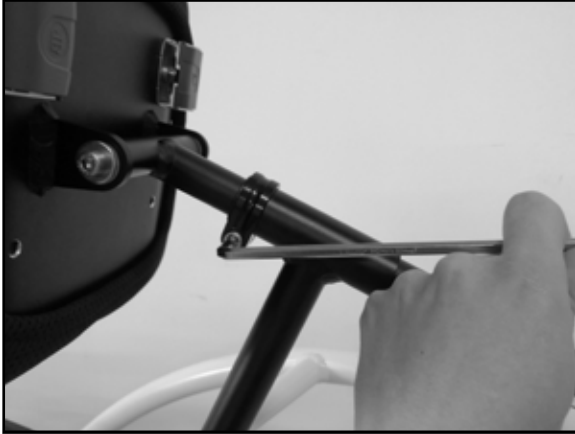
Image 11 Loosen the bolt to adjust chestplate
