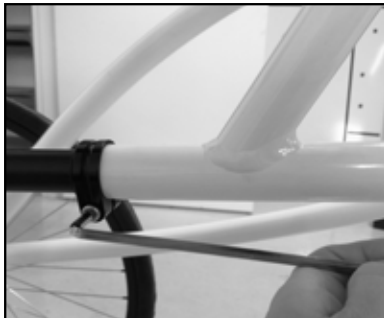
Image 5 Loosen the bolt to depth adjust
