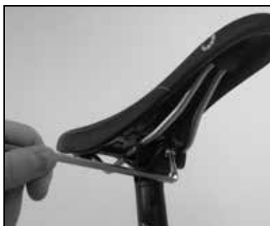
Image 8 Loosen the bolt to angle adjust
