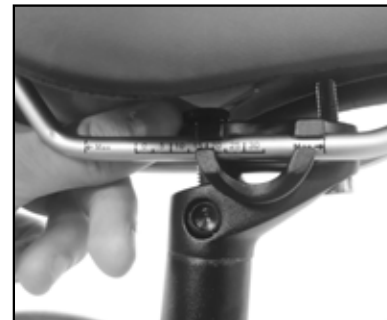
Image 9 Turn the bolt to angle adjust
