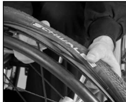
Image 18 Pull out the tube
