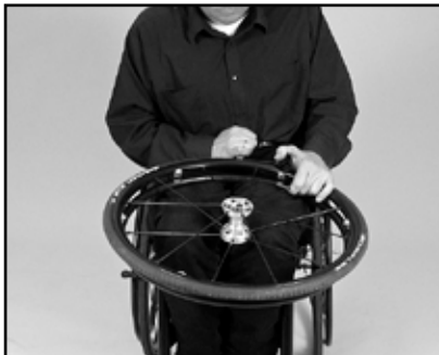
Image 17 Pull the tyre edge over the rim
