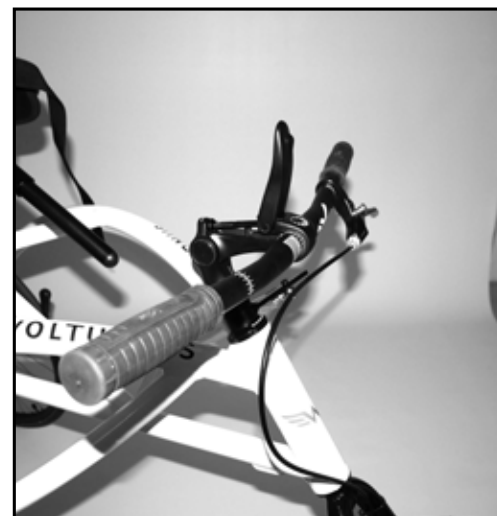
Image 10 With the tap lifted, the handlebar can rotate
