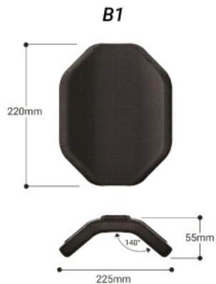
mountable on widths from 240mm to 260mm
